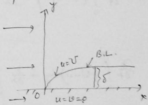
$$\Rightarrow \frac{\partial}{\partial t} \int_0^{\delta} u dy + \frac{\partial}{\partial x} \int_0^{\delta} u dy + [uv]_{y=0}^{\delta} = - \frac{1}{\rho} \frac{\partial p}{\partial x} [\gamma]_{y=0}^{\delta} + \nu \left[ \frac{\partial u}{\partial y} \right]_{y=0}^{\delta}$$
