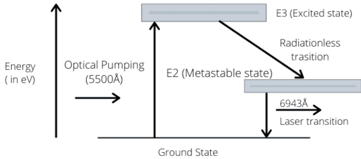
Since the state of population inversion is not a stable one, hence one or two electrons come down to ground state spontaneously. During this transition, a photon is emitted which induces stimulated emission.
