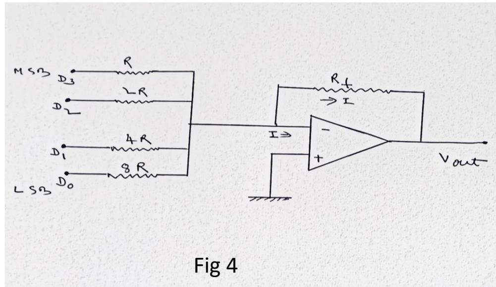
In this DAC , OPAMP is connected as an inverting amplifier and hence each input is amplified by a factor equal to the ratio of the feedback resistance divided by the resistance to which it is connected as shown in figure . The most significant bit (MSB)  $D_3$  amplified by  $\frac{R_f}{R}$  ,  $D_2$  is amplified by  $\frac{R_f}{2R}$  ,  $D_1$  is amplified by  $\frac{R_f}{4R}$  and  $D_0$ , the least significant bit (LSB) is amplified by  $\frac{R_f}{8R}$ .
